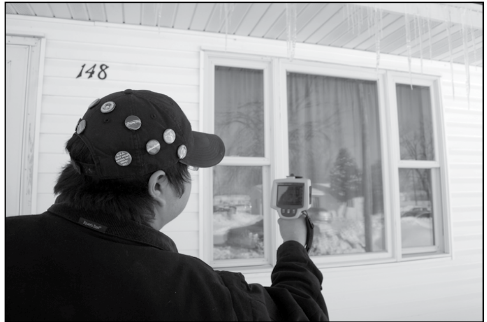
Among the weapons in the energy auditor's tool kit is the thermal imager. Students in the United Tribes Native Energy Auditor Program have been trained for its use in evaluating heating loss in buildings. United Tribes News photo Barbara Schmitt
