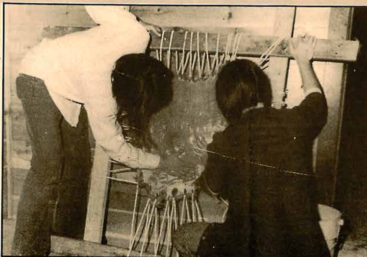
Pat Bourgeois and Mike Barthelemy rub in Neatsfoot oil. This penetrates the hide and enables the breakdown of the pores.
